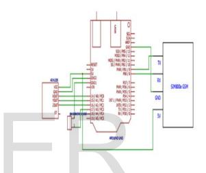
Fig. 3. The circuit diagram for fall detection system
